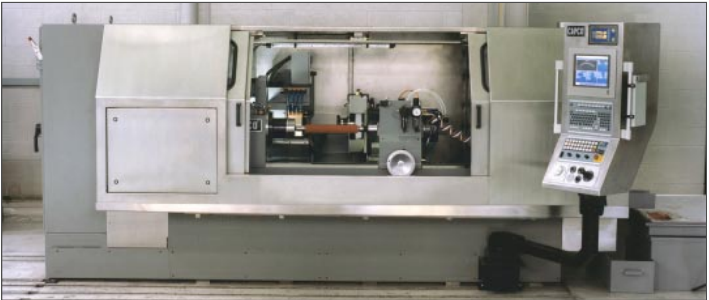
The Capco® SuperGrinder™ will be the primary machine to grind the highly accurate rolls for the newest Heidelberg digital printing presses.
